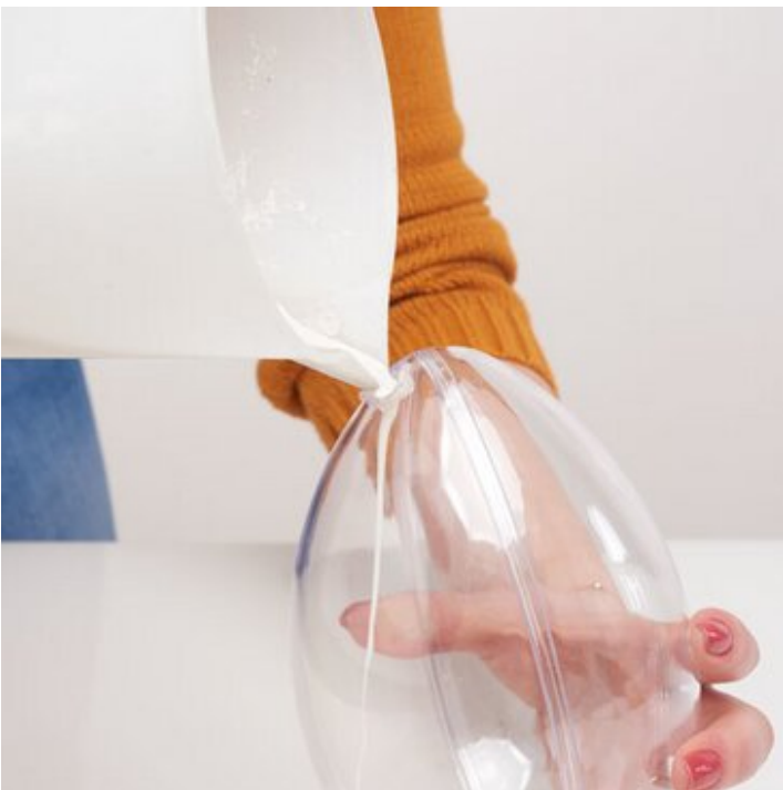
3. Pour the casting compound into the tightly closed Acrylic egg
